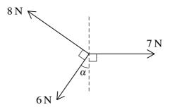
Coplanar forces of magnitudes 7 N, 6 N and 8 N act at a point in the directions shown in the diagram. Given that  $\sin \alpha = \frac{3}{5}$ , find the magnitude and direction of the resultant of the three forces. [5]
